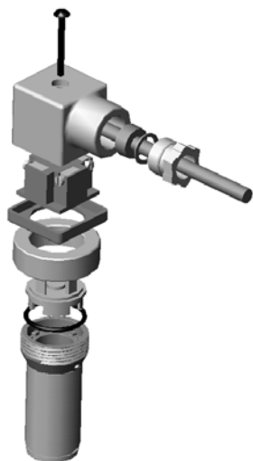
Figure 1 - Exploded view of the connector
